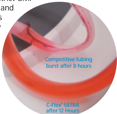
In a 24-hour pumping trial, competitive tubing failed at less than 12 hours.
